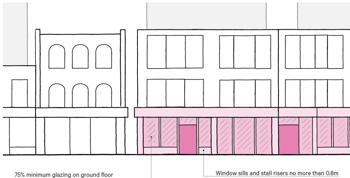
Figure 2. Glazing requirements – Urban Setting
